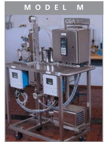
Laboratory-scale feasibility study of ceramic, spiral or hollow fiber MF or UF
