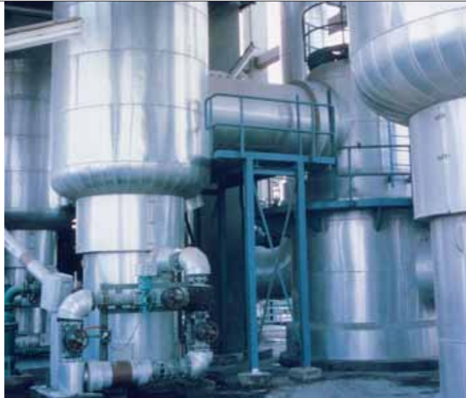
Salt crystallizer; modified FC-type
