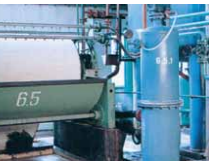
Vacuum filter for citrate extraction
