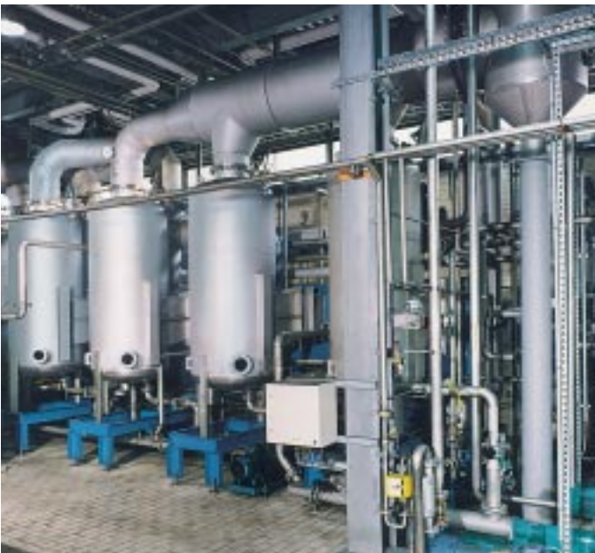
Multiple-effect plate evaporation plant for fructose. Evaporation rate: 16 t/hr
